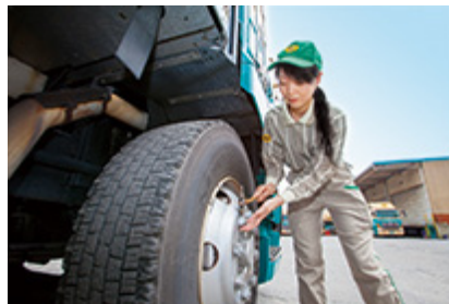
Inspection of wheel bolts prior to leaving
